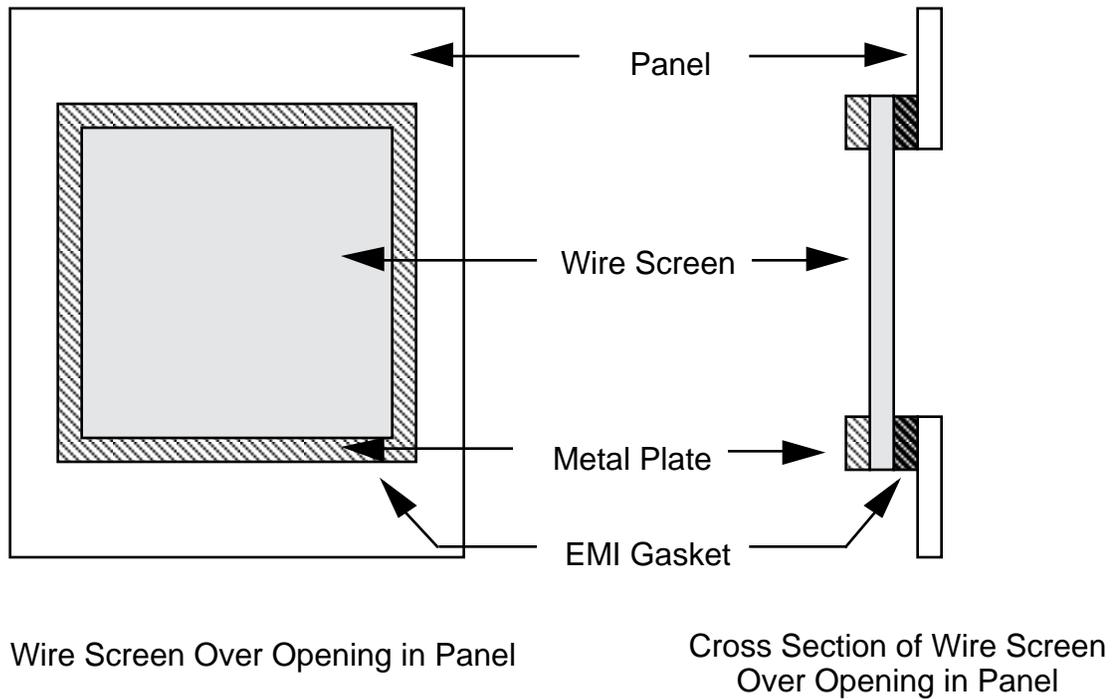
Figure 3-30. Examples of uses for conductive gaskets.
