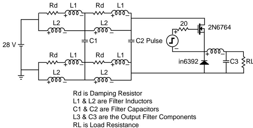
Figure 4-1. Buck regulator power supply with two-stage filter.
