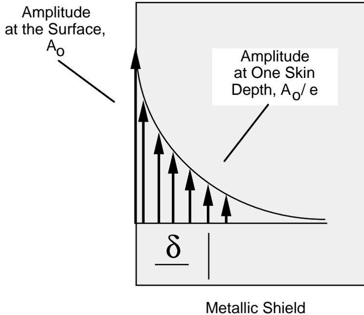
Figure 3-23. Schematic definition of skin depth.
