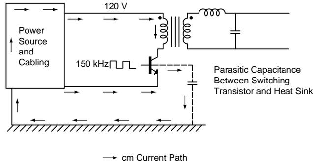
Figure 4-7. Switched-mode power supply with CM noise path.
