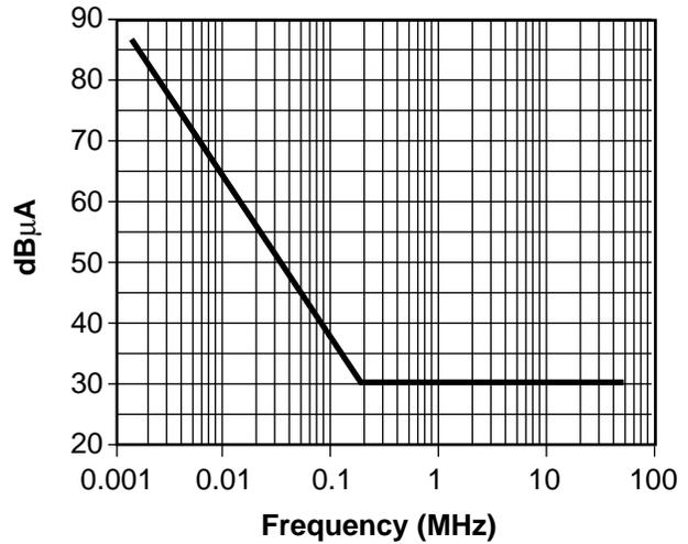
Figure 5-15.2. CE current to limit RE from cables.
