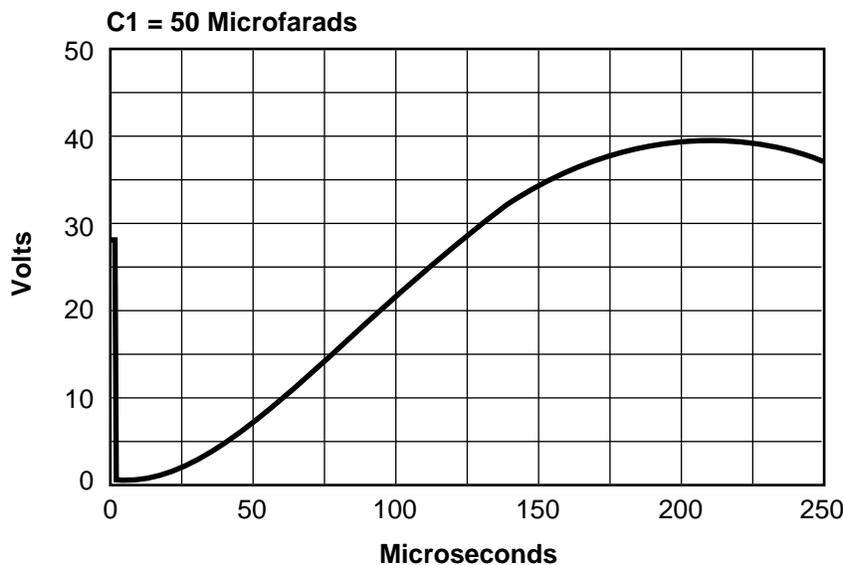
Figure 4-12(b). Predicted turn-on transients (50  $\mu$ F).
