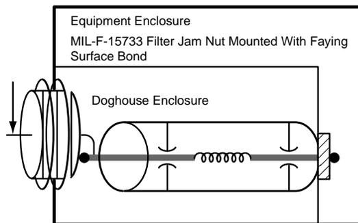
Connector Shell Typically Jam Nut Mounted Enclosure and Doghouse, Ensuring Faying Surface Bonds to All Three Components (Power Return Thru Structure and Equipment Chassis)
