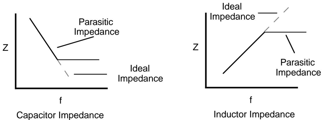
Figure 3-14. Inductor and capacitor impedance.
