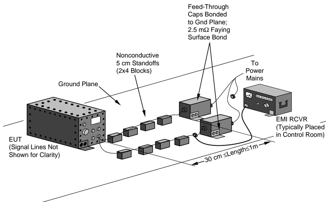
Figure 5-1. Full compliance current CE test setup.
