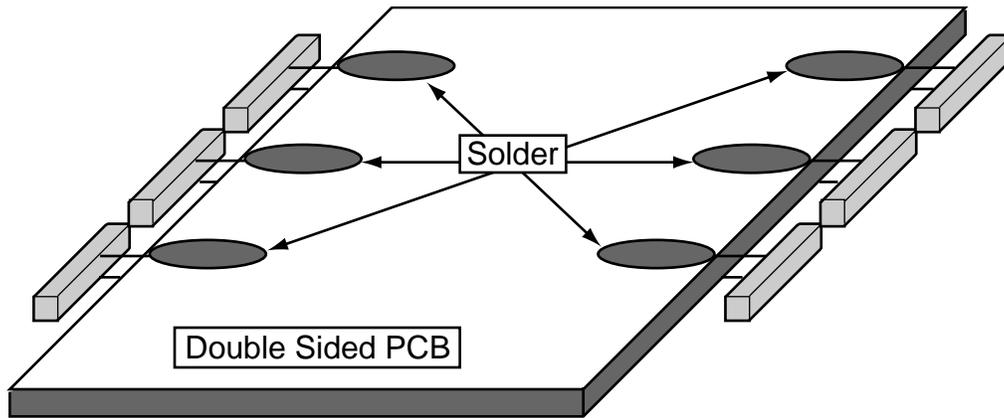
Reverse Side of PCB Is Identical to That Shown; Caps Should Be Up Against PCB Side, Maximum Amount of Cap Lead Should Be Soldered to Plane in Order to Minimize Lead Inductance
