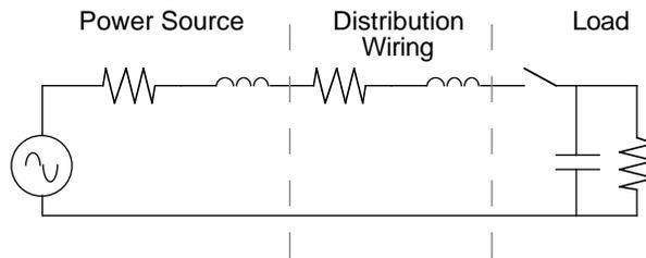
Figure 5-17.1. Model of electrical power distribution system.
