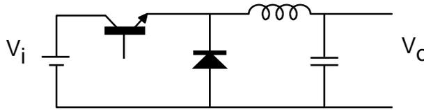
Figure 3-36. Buck converter topology.
