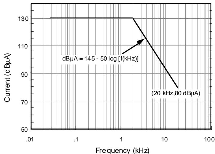
Figure 2-1. CE01 limit for Spacelab 28-Vdc loads.
