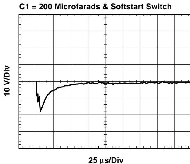
Figure 4-14. Transient test data using soft-start switch.
