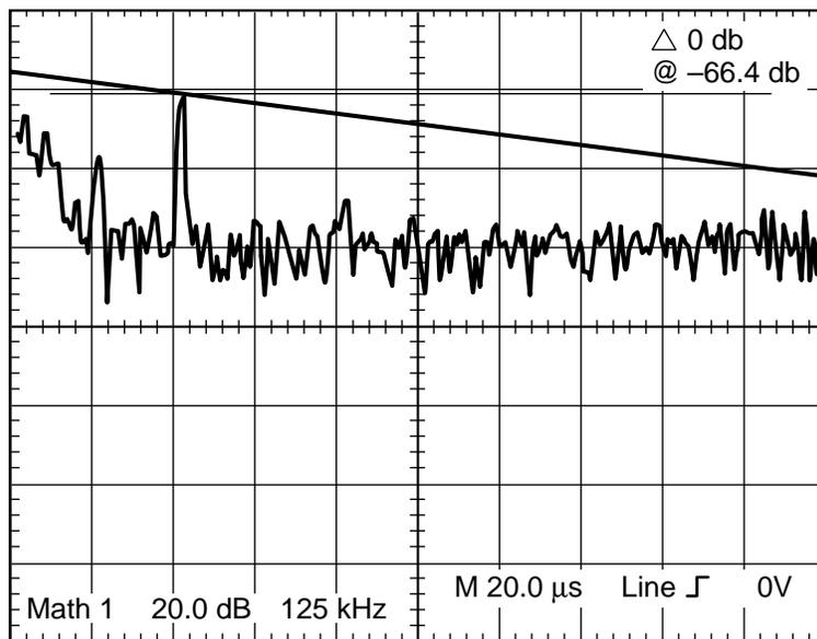
Figure 5-13.5(b). CM filtering: as above plus 20- $\mu$ F line-line X-capacitance, for DM filtering, 28 VRTN, low frequency (Y-axis 20 dB/div, compare amplitudes to limit line; X-axis is linear, 125 kHz/div, starting at dc).
