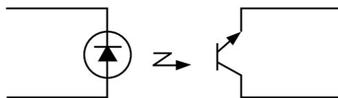
Figure 3-22. Opto-isolator schematic.
