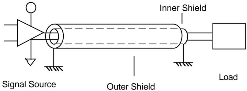
Outer and Inner Shields are Grounded at One End and Ungrounded at the Other End. The Two Shields are Isolated From Each Other at DC. At High Frequencies, the Capacitance Between the Inner and Outer Shield is Such That the Shield Acts as if it Were Electrically Grounded at Both Ends. This is Effective Against High Frequency Radiated Fields.
