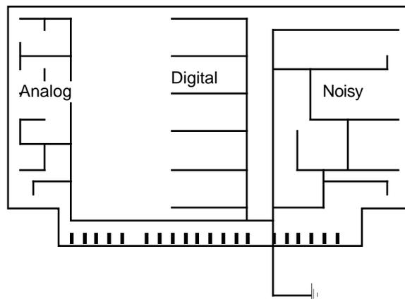
Figure 3-48. Separate ground systems.
