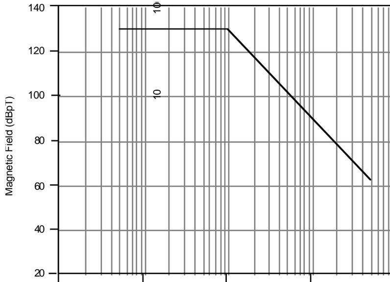
Figure 2-9. RE04 limit of MSFC-SPEC-521B.
