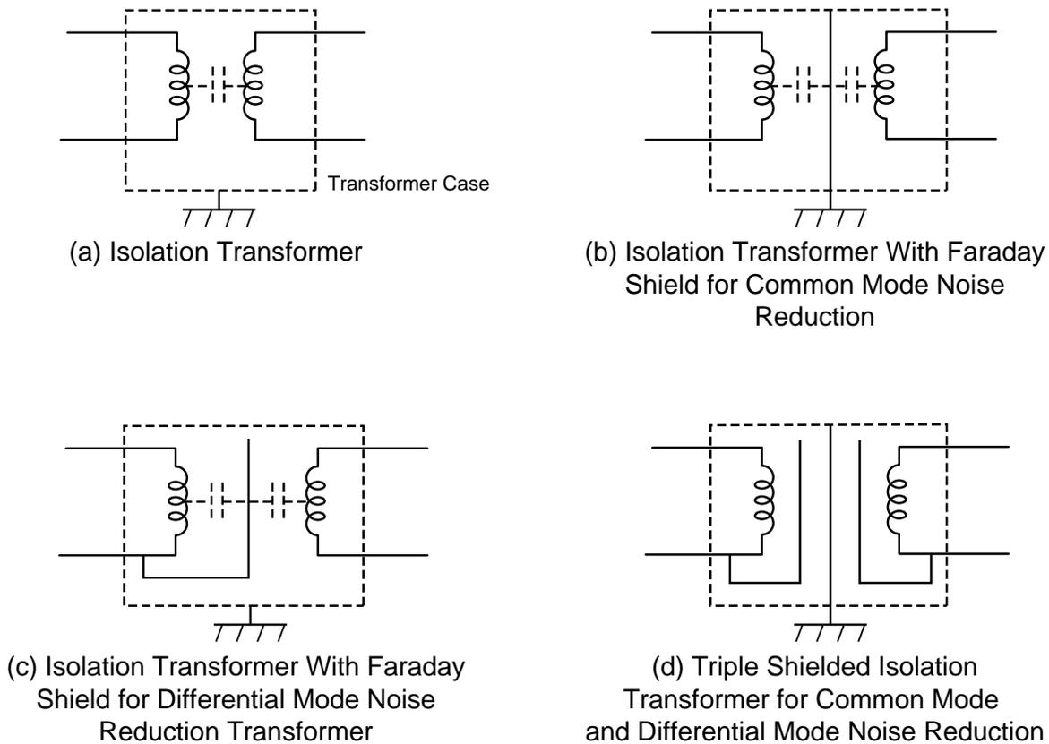
Figure 3-21. Isolation transformer configurations.
