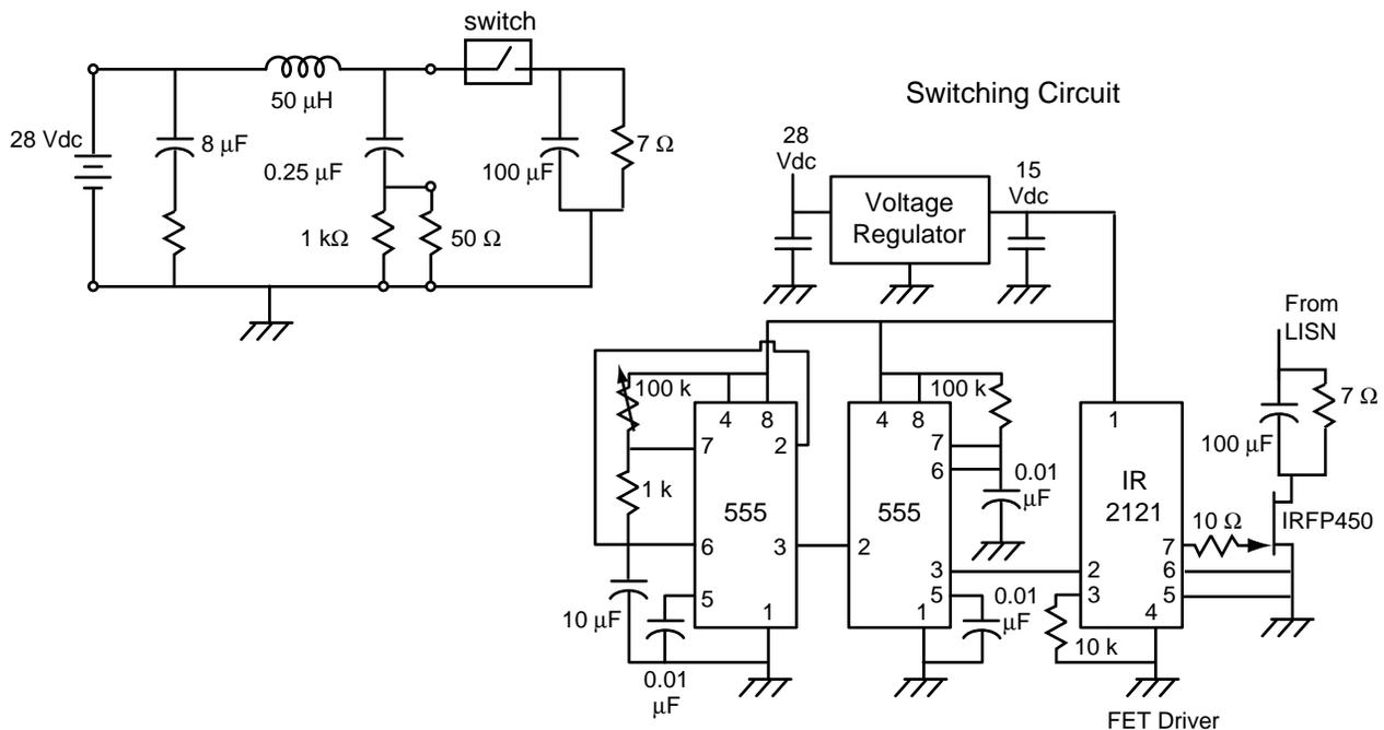
Figure 5-17.5. Transient generating circuit for 28-Vdc loads.
