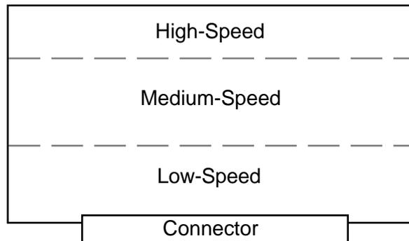
High-Speed Circuitry Has No I/O External to Board
