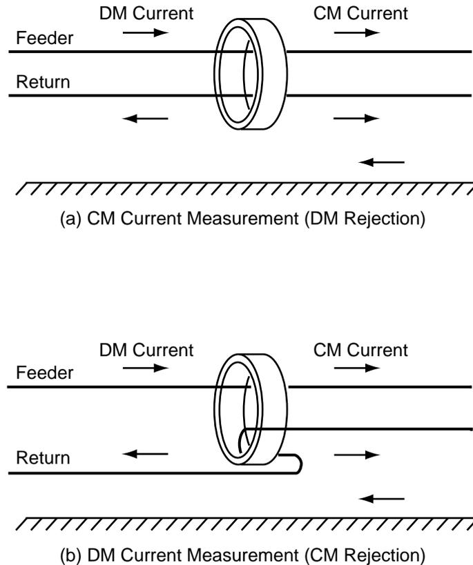
Figure 5-12. Mode selection/rejection with current probes.
