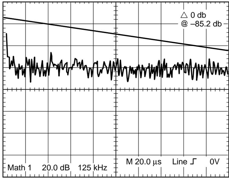
Figure 5-13.6(a). CM filter plus complete DM filter; as above plus 100- $\mu$ H choke in 28-Vdc line, 28-Vdc input, low frequency (Y-axis 20 dB/div, compare amplitudes to limit line; X-axis is linear, 125 kHz/div, starting at dc).
