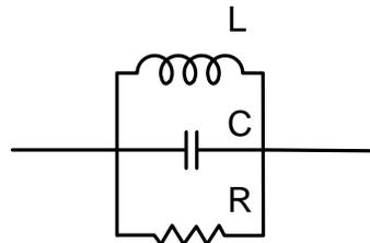
Figure 4-15(b). Damping with parallel resistance.
