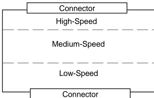
Figure 3-9(d). Suggested board layout with separate connectors.
