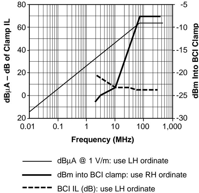
Figure 5-16.1. Converting 1-V/m field to bulk current drive.
