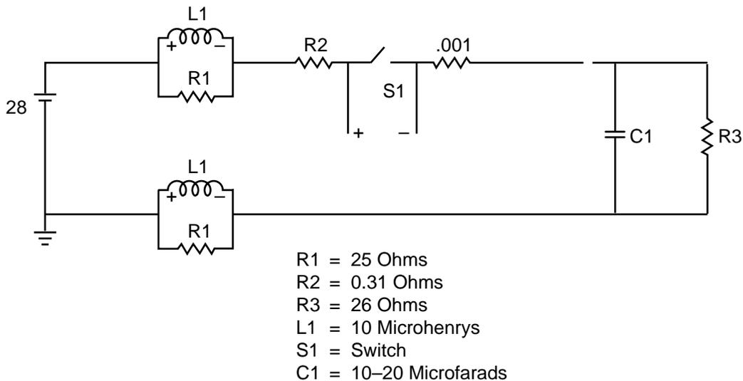
Figure 4-11. Transient test setup.
