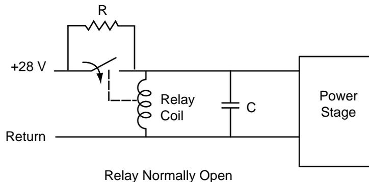
Figure 4-9. Soft-start switch using relay.
