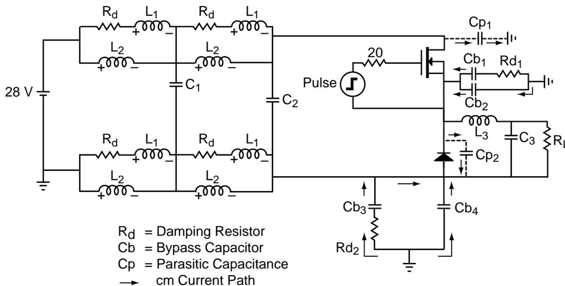
Figure 4-2. Buck regulator power supply with parasitic capacitances.
