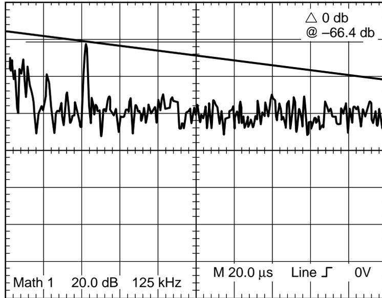
Figure 5-13.5(a). CM filtering: as above plus 20- $\mu$ F line-line X-capacitance, for DM filtering, 28-Vdc input, low frequency (Y-axis 20 dB/div, compare amplitudes to limit line; X-axis is linear, 125 kHz/div, starting at dc).
