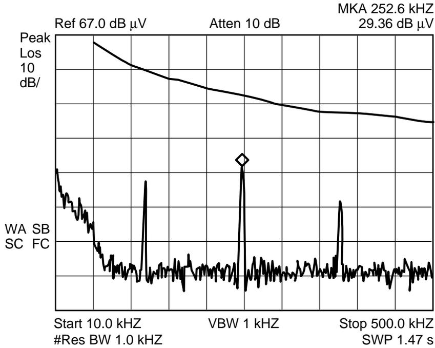
Figure 5-13.8(c). Verification using EMC spectrum analyzer, 28 VRTN, low frequency.
