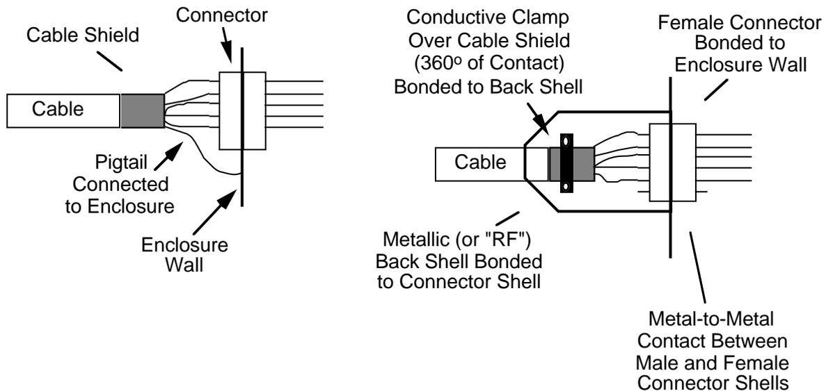
Figure 3-31. Pigtail and RF backshell terminations.
