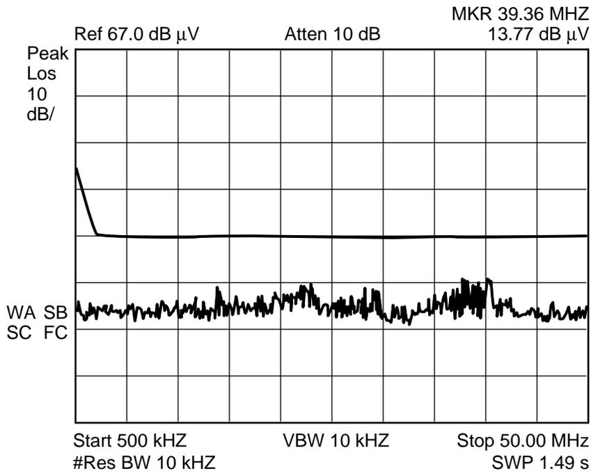
Figure 5-13.8(d). Verification using EMC spectrum analyzer, 28 VRTN, high frequency.
