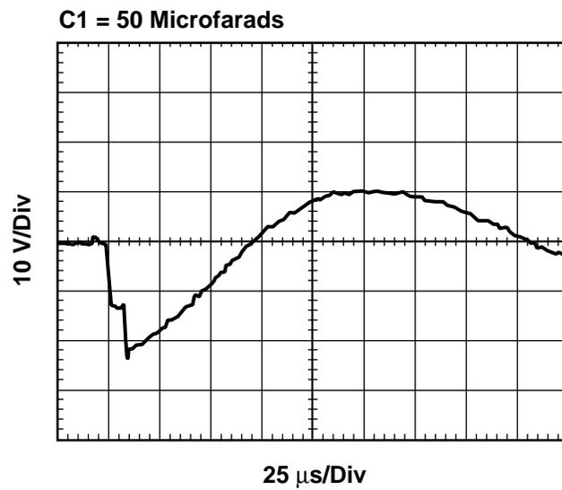
Figure 4-13(b). Turn-on transient test data (50  $\mu$ F).
