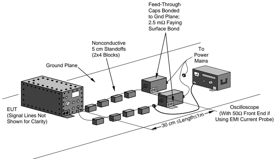
Figure 5-2. Diagnostic CE test setup.
