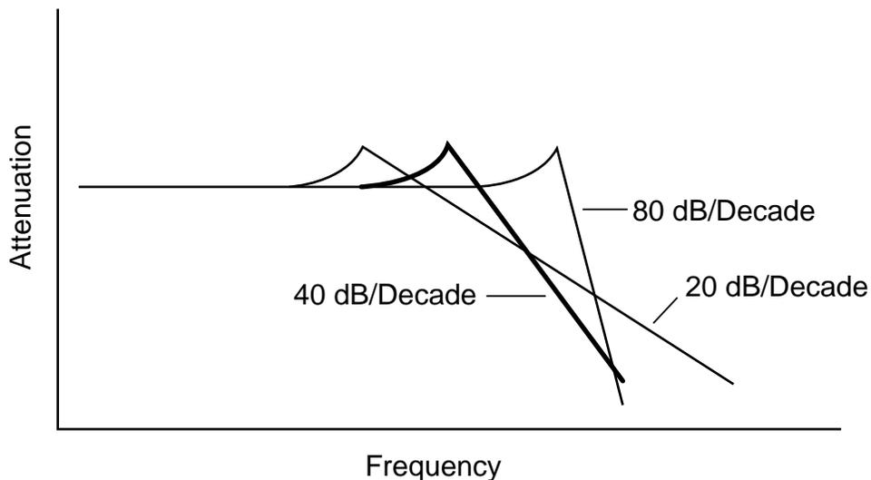
Figure 4-6. Bode plot for three LC filters.
