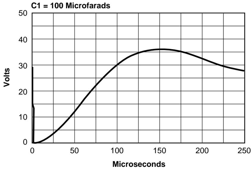
Figure 4-12(c). Predicted turn-on transients (100  $\mu$ F).
