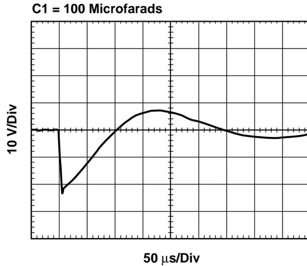
Figure 4-13(c). Turn-on transient test data (100  $\mu$ F).
