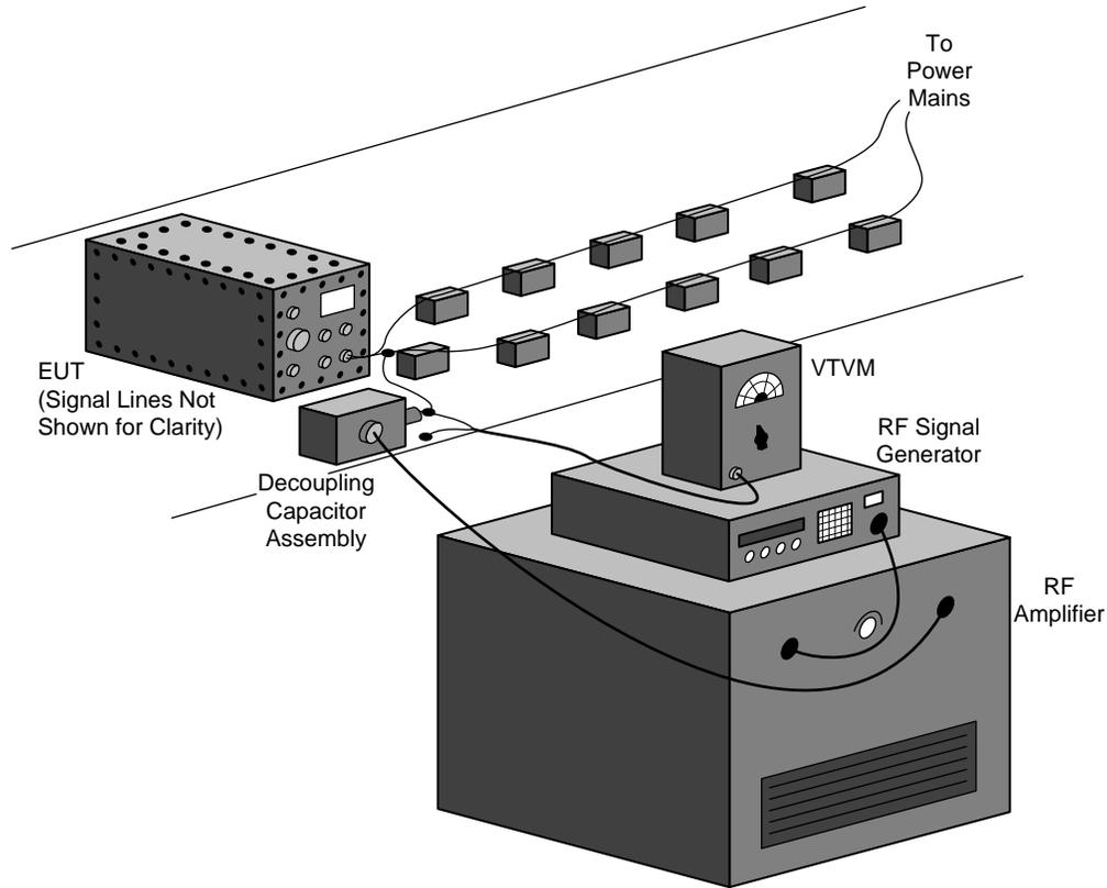
Fig 2-12. CS02 test setup.
