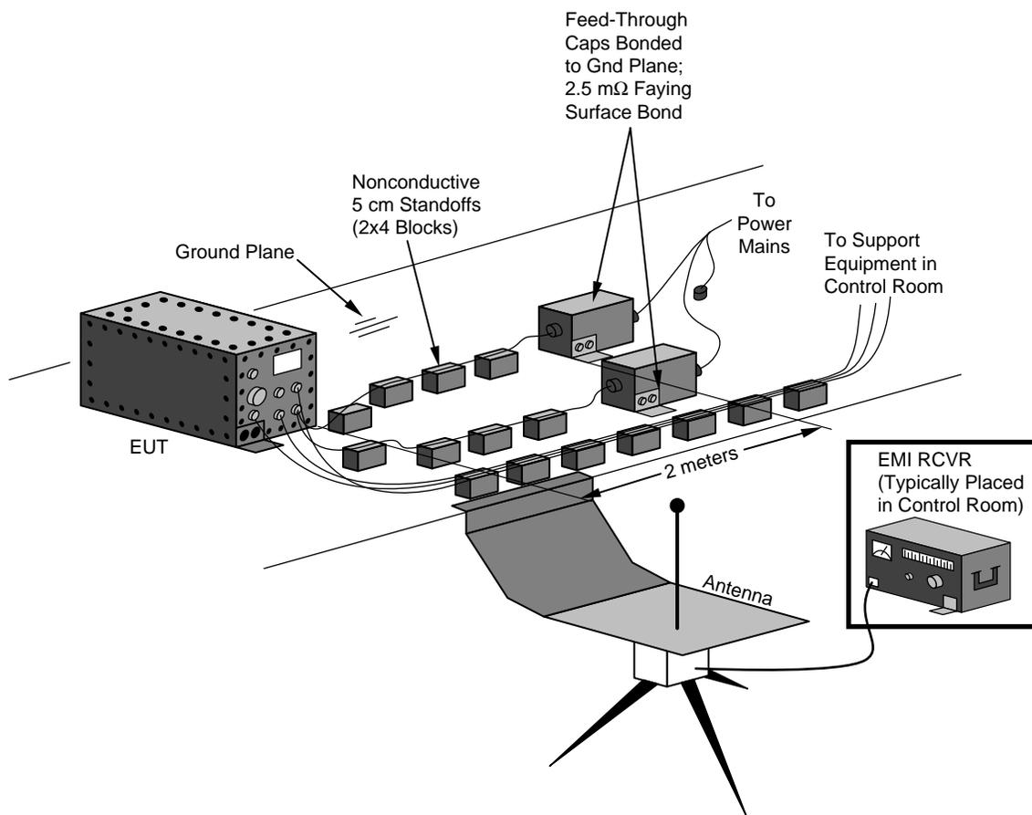
Figure 2-8. RE02 test setup, 41-in rod antenna test (0.01 to 30 MHz)
