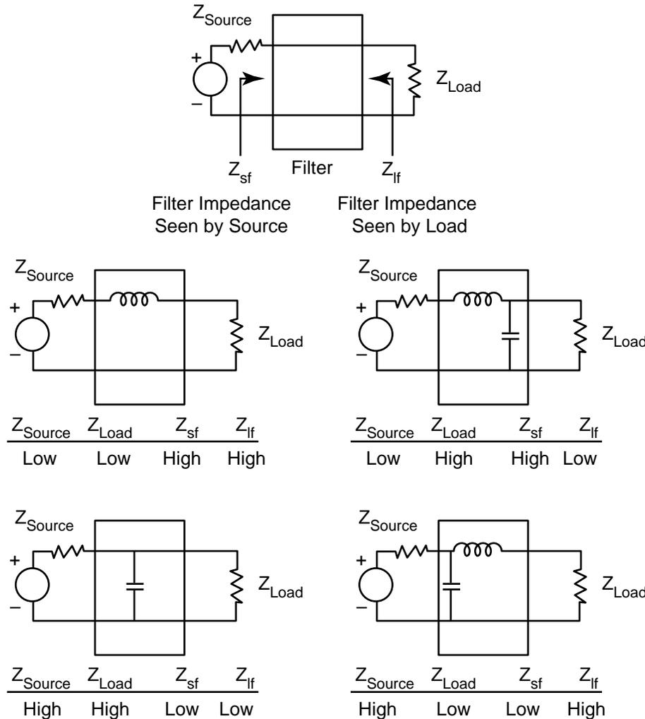
Figure 3-15. Filter configuration examples.<sup>3-7</sup>
