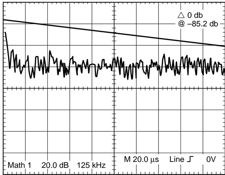
Figure 5-13.6(b). CM filter plus complete DM filter; as above plus 100- $\mu$ H choke in 28-Vdc line, 28 VRTN, low frequency (Y-axis 20 dB/div, compare amplitudes to limit line; X-axis is linear, 125 kHz/div, starting at dc).
