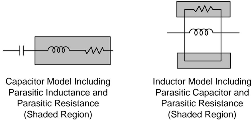
Figure 3-13. Capacitor and inductor models including parasitics.
