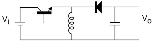
Figure 3-38. Buck-boost converter topology.
