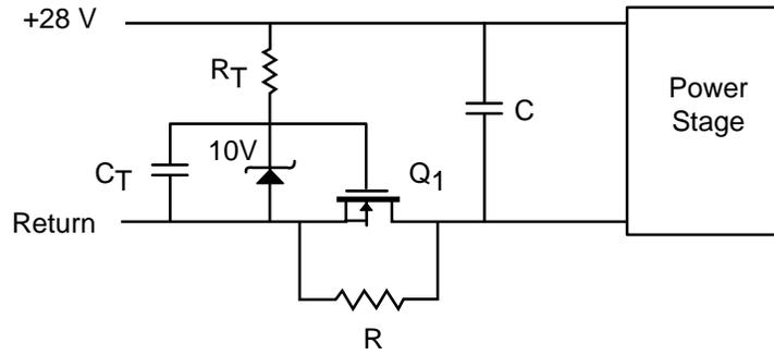
Figure 4-10. Soft-start switch using MOSFET.
