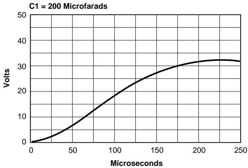
Figure 4-12(d). Predicted turn-on transients (200  $\mu$ F).
