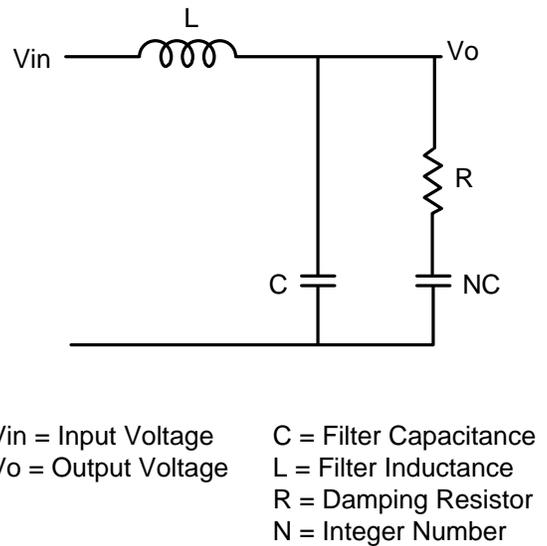
Figure 4-16(b). Damping resistor for parallel capacitors.
