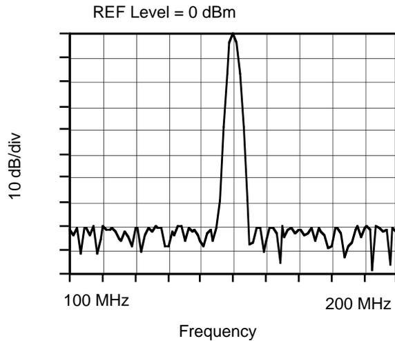
Figure 1-7. Spectrum analyzer log signal display.
