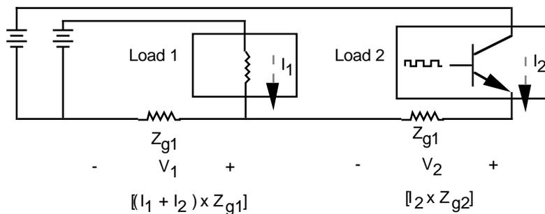
Figure 3-49. Common-impedance coupling.
