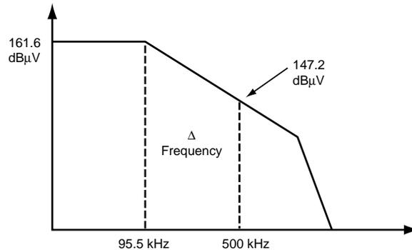
Figure 4-8. Frequency domain spectrum envelope.
