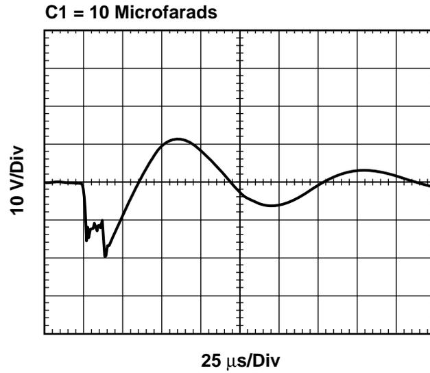
Figure 4-13(a). Turn-on transient test data (10  $\mu$ F).
