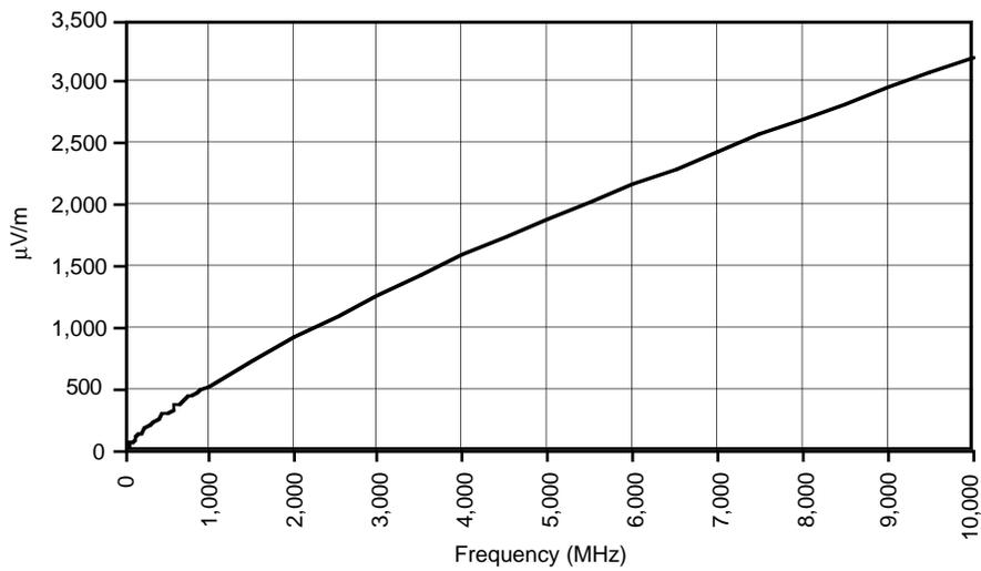
Figure 1-6. MIL-STD-461C RE02, part 2 with linear axes.
