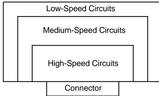
Figure 3-9(b). Suggested board layout for multispeed circuits.
