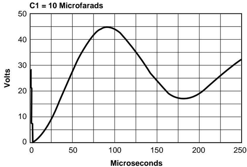
Figure 4-12(a). Predicted turn-on transients (10  $\mu$ F).
