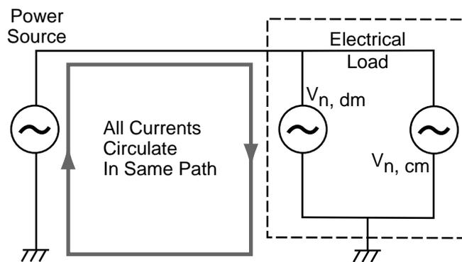
Figure 5-9. Noise current circulation in structure return bus.
